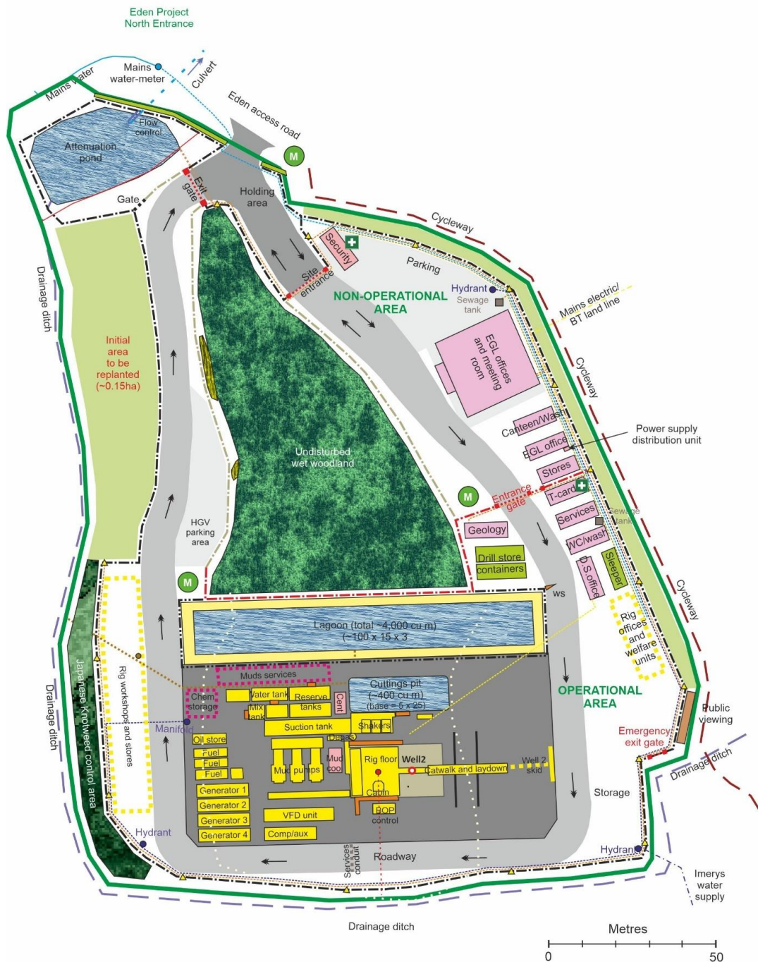
Proposed Layout of the Deep Geothermal Site at the Eden Project, Cornwall during the Construction Phase
