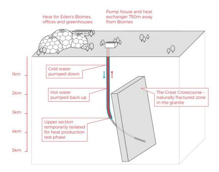
Phase 1 of Eden Geothermal Project
